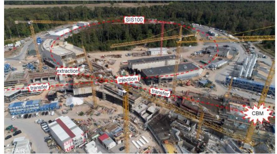
SIS100: synchrotron ring of magnetic rigidity 100 Tm
