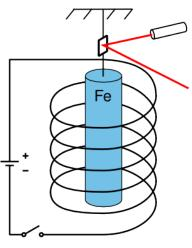
Electron spins get aligned in external magnetic field which is compensated by rotation of the ferromagnetic material.
